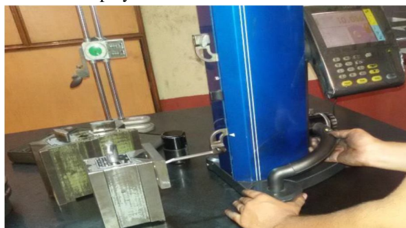
Fig-4.2:- Trimos instrument using for our project
